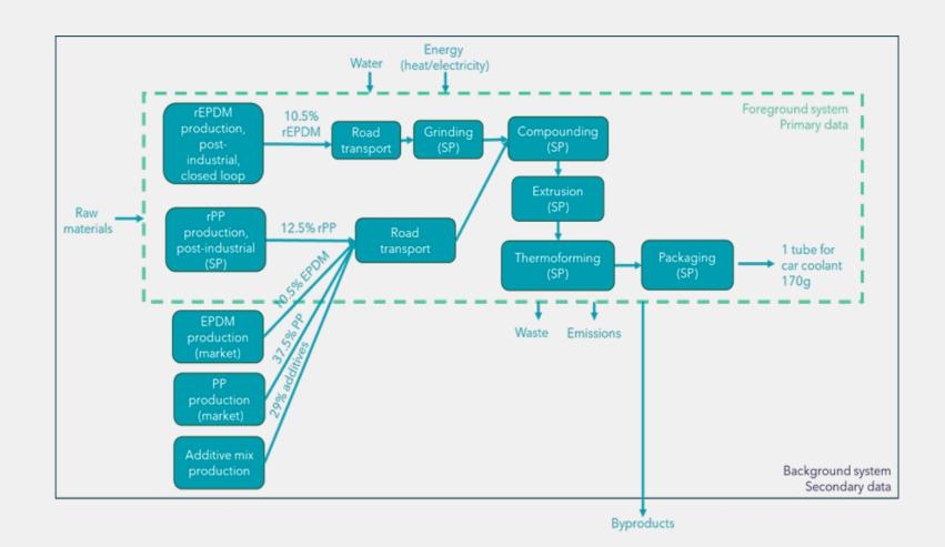
Figure 12. System Boundaries of the Demo 2 LCA model
