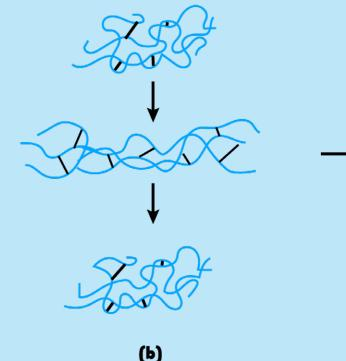
Figure 9. Difference between (a) Thermoplastic and (b) Elastomer polymer chains.
