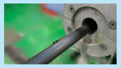
Figure 10. Extrusion of TPV material
