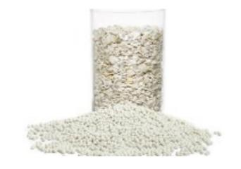
Figure 15 - rHIPS flakes (before extrusion) and granules (after extrusion).
