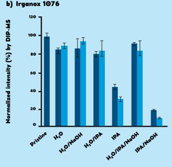
both 2500 and 25000 ppm model compounds using H2O/IPA/NaOH. Moreover, based on differential scanning calorimetry, 1H NMR, and size exclusion chromatography analyses, no significant polymer degradation was observed due to any of the applied extraction conditions. The main challenge was the observation that the extraction efficiency was highly dependent on the particle size, and cryo-grinding was necessary to achieve high BFR removal<sup>11</sup>.
