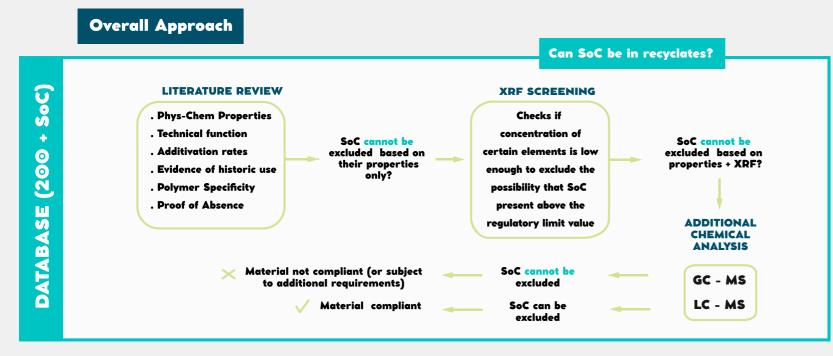
• X-Ray Fluorescence (XRF) at the recycler's site to detect elements linked to regulated substances.
