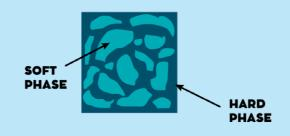
Figure 8. EPDM/PP cured blend (TPV) morphology.
