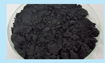
Figure 20. Recyclate produced by grinding the end of life washing machines
