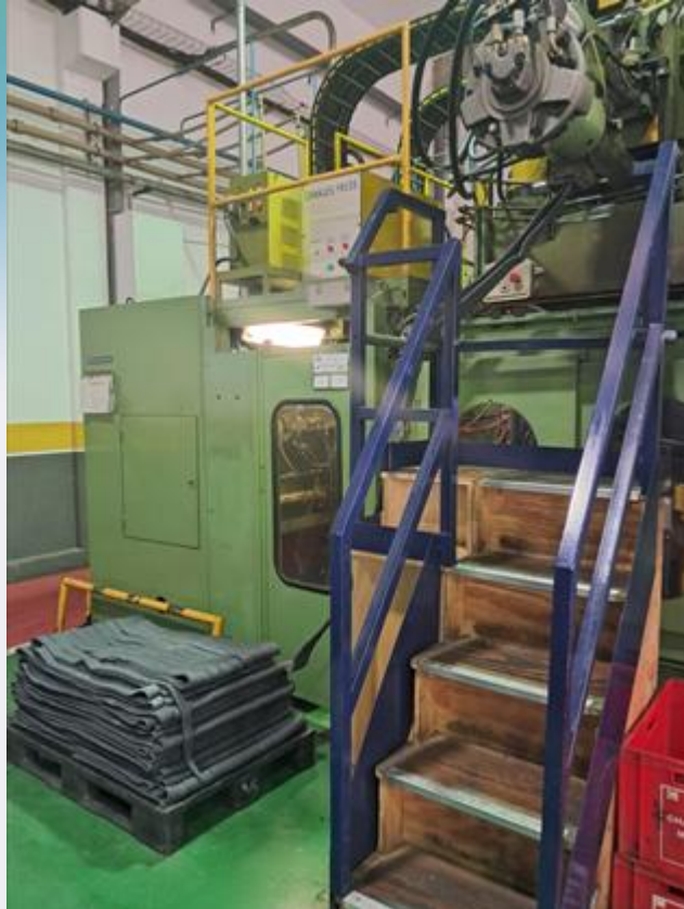
Injection machine used for the production of the demonstrators
