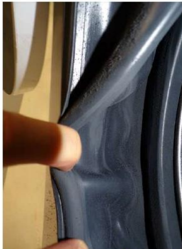
Wear of the part after several hours of test but still the hole has not appeared
