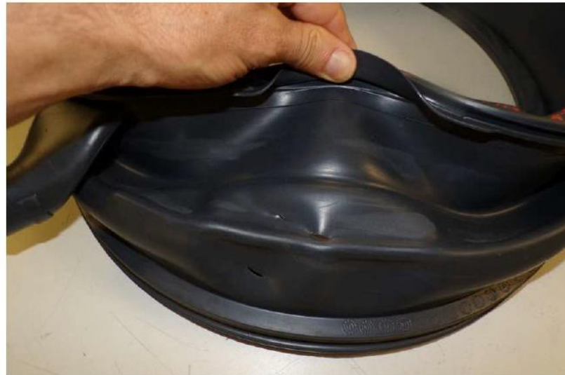
Hole produced as a consequence of the durability test
