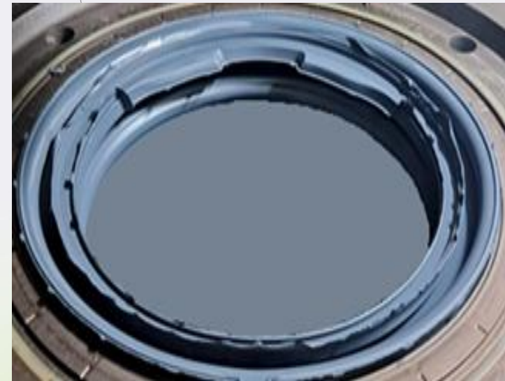
Mold used for the production of the demonstrators
